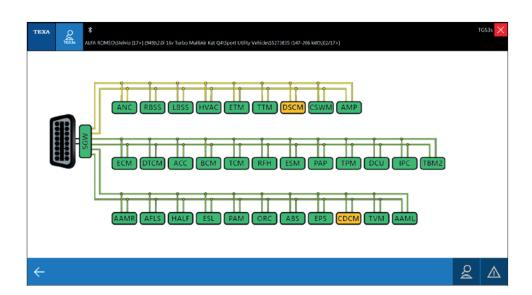
Through this screen you can get a simplified and clear view of the vehicle's communication line and of the control units that have errors.
